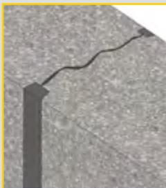
Aligned keyways create a controlled crack to introduce Krystol technology through two external waterstops that ensure permanent waterproofing protection.
